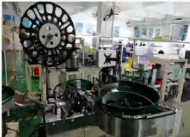
RJ45 connector automatic assembly line
