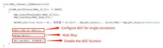
3.2.2 Software trigger Precautions for enabling ADON to perform external events twice in a row
